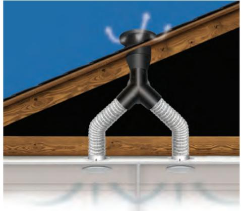
The best way to ventilate bathrooms is to vent it through the roof cavity
